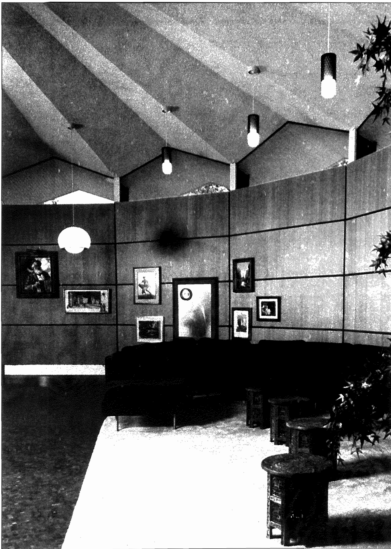
With glass above and below, the curved, silk-paneled wall seems to float. More than 183,000 tiny squares of walnut cover the floor in the living and dining rooms.
